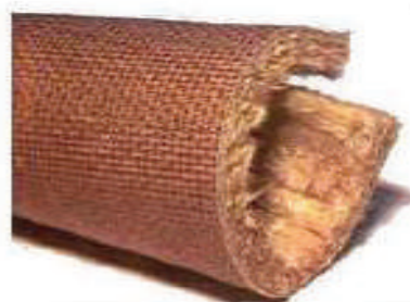
0.5-INCH THICK NON-WOVEN INSULATION MATERIAL, LAMINATED
